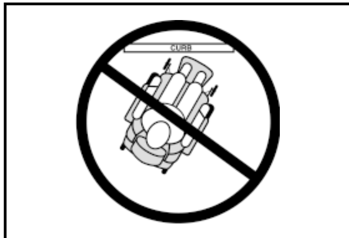
Figure 3. Incorrect Curb Approach
